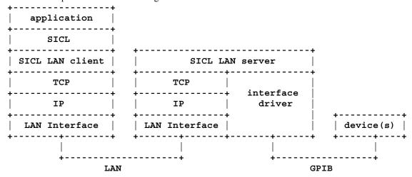
Once the software has been configured, however, a programmer does not need to be concerned with the fine details of networking operation; he or she can open up a session with an instrument on the E2050 or LAN server software by invoking an "iopen" call with the appropriate address. For example:
