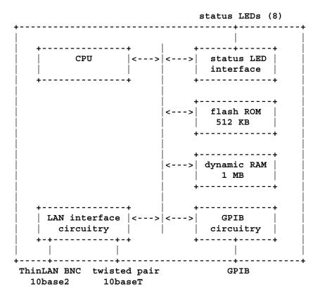
A single E2050 can support up to 14 GPIB instruments connected to its GPIB; up to 10 client transactions can be connected at any single time. (The default GPIB address of the E2050 itself is 21.) The E2050 *cannot* be a non-system controller!
