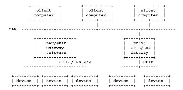
The client computer deals with the servers through the SICL LAN software. The operations are based on the standard TCP/IP protocols and can be diagrammed as follows:
